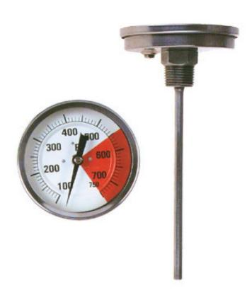
BACK CONNECTED -3". All welded sus 304 stainless steel construction of this instrument provides the durability for work in corrosive environments and ensures long service life. The instrument has been designed to handle the accurate temperature measurements of industrial and laboratory applications. A hex nut located at the rear of the case is used for recalibrating if necessary.
